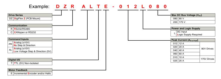
DigiFlex® Performance $^{\text{TM}}$  series of products are available in many configurations. Note that not all possible part number combinations are offered as standard drives. All models listed in the selection tables of the website are readily available, standard product offerings.
